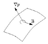
B lines is in the surface of p = const. In equilibrium isobaric surface are "magnetic surface"
